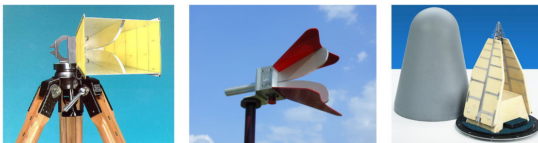
Figure 3.19 Antennas used in the simulations from left to right: double-ridged waveguide horn, the special double-ridged waveguide horn, and the log-periodical antenna with radome.
