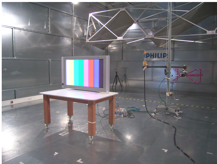
Figure 1.3 Test configuration in the reverberation chamber at the Philips EMC center.
