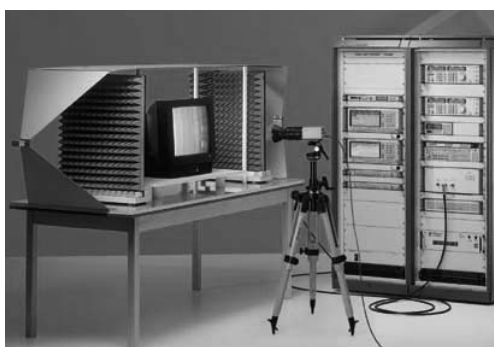
Figure 6.1 TEM waveguide (Jacky) immunity test configuration.
